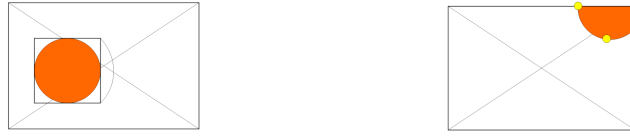
Figure 3.1: Cases of Ball Recognition. Dots on the edge show vertexes of a inscribed triangle. The diameter of the ball is calculated by using these vertexes.
